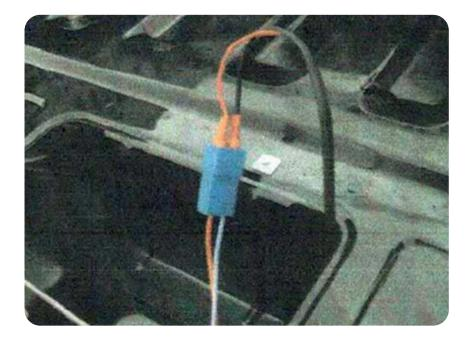
**7.**/Feed Cables out of tailgate and strap tight using cable ties. Feed out towards the side the fuel filler cap is.
