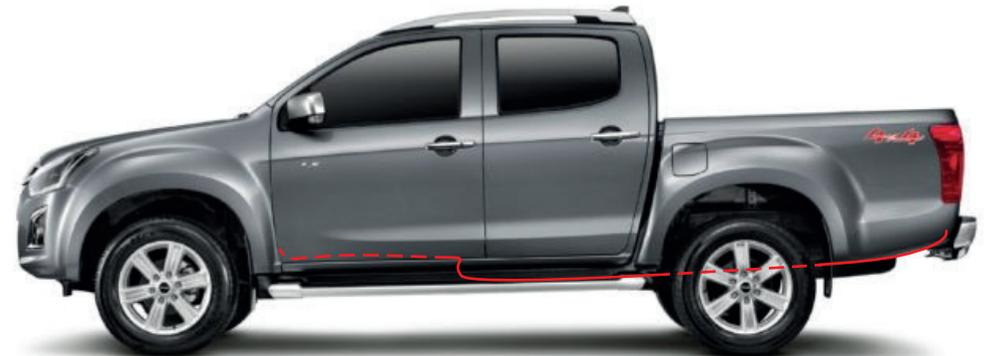
Remove the door sill guard on the driver's side to expose the vehicle's wiring loom
