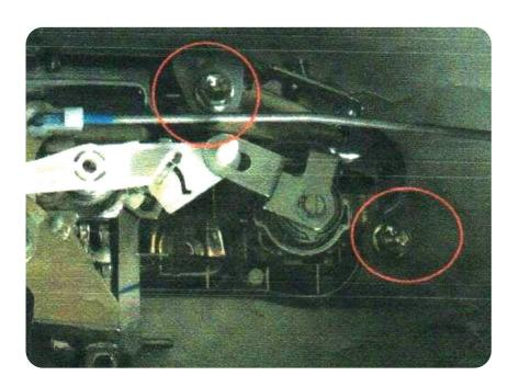
**5.**/ Remove key barrel lock (press the spring clip together and simply pull out).
