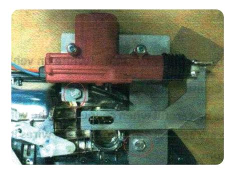
**7.**/ Refit key barrel. Simply slide back into position. Ensure you slide through power lock and into the trucks lock mechanism.
