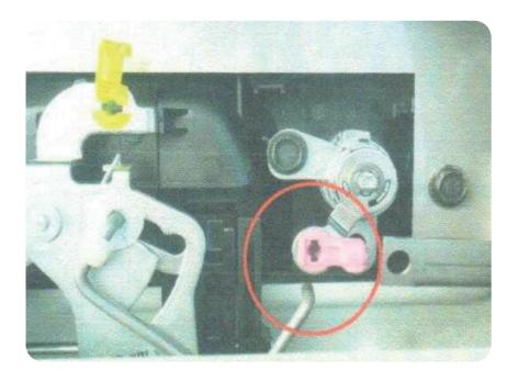
7./ Attach the StarLock to the vehicle's lock barrel (use new clip provided). Re-insert the locking rod into new clip
