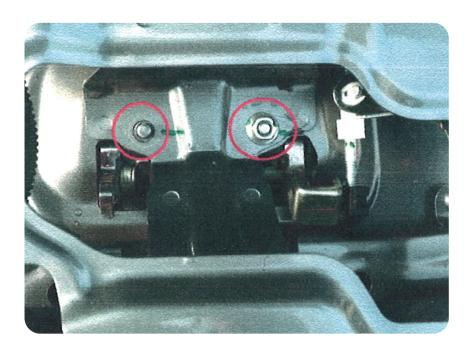
**5.**/ Install the base plate and actuator kit using the bolts removed in step 4.
