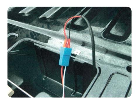
**7.**/ Feed cable out of the tailgate on passenger's side. Use convoluted tubing provided to protect cable.
