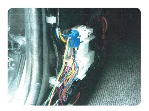
**10.**/Connect the central locking kit into the vehicle central locking loom
