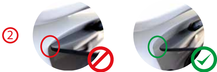
② A space is needed at the top of the tailgate between the glass and the Hard Top
