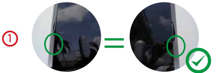
① The space between Hatchback and Canopy must be identical on each side
